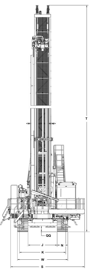
'Approximate shipping dimensions for crated PV-275 (actual dimensions will vary based on rig configuration).
