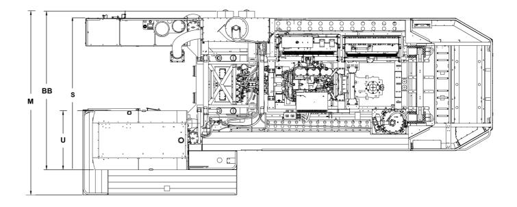
Width – overall with dust collector overhang
